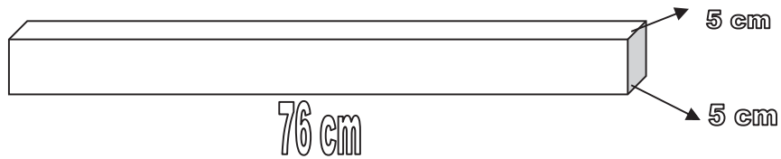
Gambar 1. Contoh Uji berdasarkan American Society for Testing and Materials (ASTM) D 143-94.
