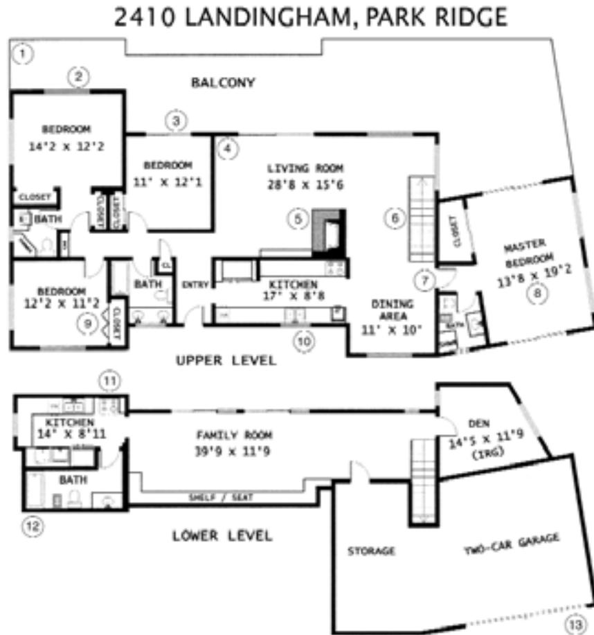
**Figure 7-12:** This house floor plan uses only a few of the many architectural drawing symbols
